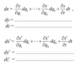
The displacements  $dq_1, \ldots, dq_h$  imply that none of the contact have slippage, so the two displacements dx, dy, dz and dx', dy', dz' agree in magnitude and direction. In particular, the same thing will be true for the h + 1 displacements that are obtained by varying  $q_1, \ldots, q_h, t$  separately, which are displacements that are pair-wise identical in the common tangent plane to the two bodies S and S' considered.
